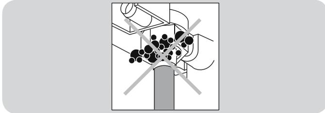
Apply pressure to device and test the joints using leak detection spray. No bubbles should form.
