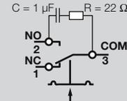
In the case of high humidity or aggressive gas components ( $H_2S$ ), we recommend using a pressure switch with gold contact due to its higher resistance to corrosion. Closed-circuit current monitoring is recommended under difficult operating conditions.
