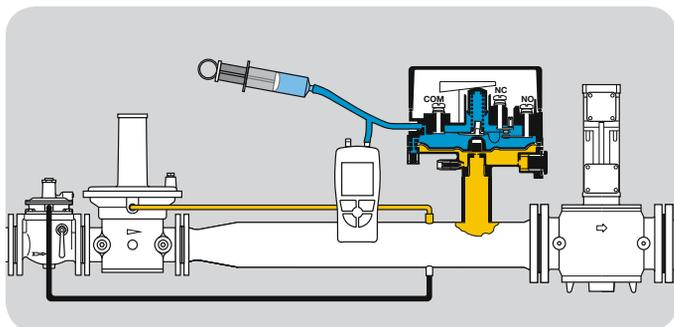
the pressure is measured at the test point. In this example, it is 55 mbar. Then the open 1/8" port, which is usually used to measure atmospheric pressure, is attached to a syringe and connected measuring instrument. The plunger is then pushed in slowly and the reaction of the system is observed. If the pressure is around 15 mbar ( $p_s = 55 - 15 = 40$  mbar), the DG should switch off (COM-NC) and the system should shut down.
