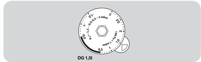
**Test:** turn hand wheel in the "Plus" direction as far as it will go (signal at COM-NO), then turn the hand wheel in the "Minus" direction until the signal changes to COM-NC (according to details on template). When simulated in a laboratory, this test produces the following results: signal at COM-NC (switch-off point) = 1.2 mbar, turn hand wheel back, switch-on point = 1.5 mbar.
